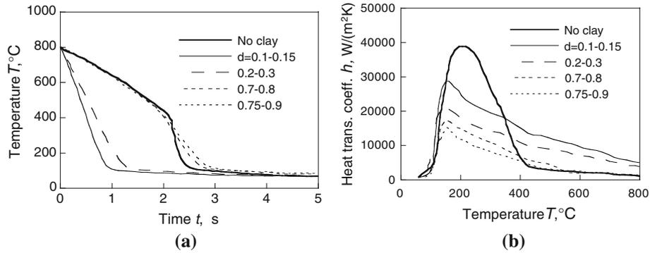
**Fig. 11** Cooling curves depending on coated clay thickness. **a** Cooling curves depending on the thickness of clay; **b** Identified Heat transfer coefficient
