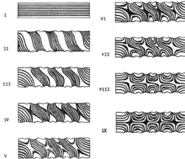
**Fig. 6** Formation of weld pattern by twisting
