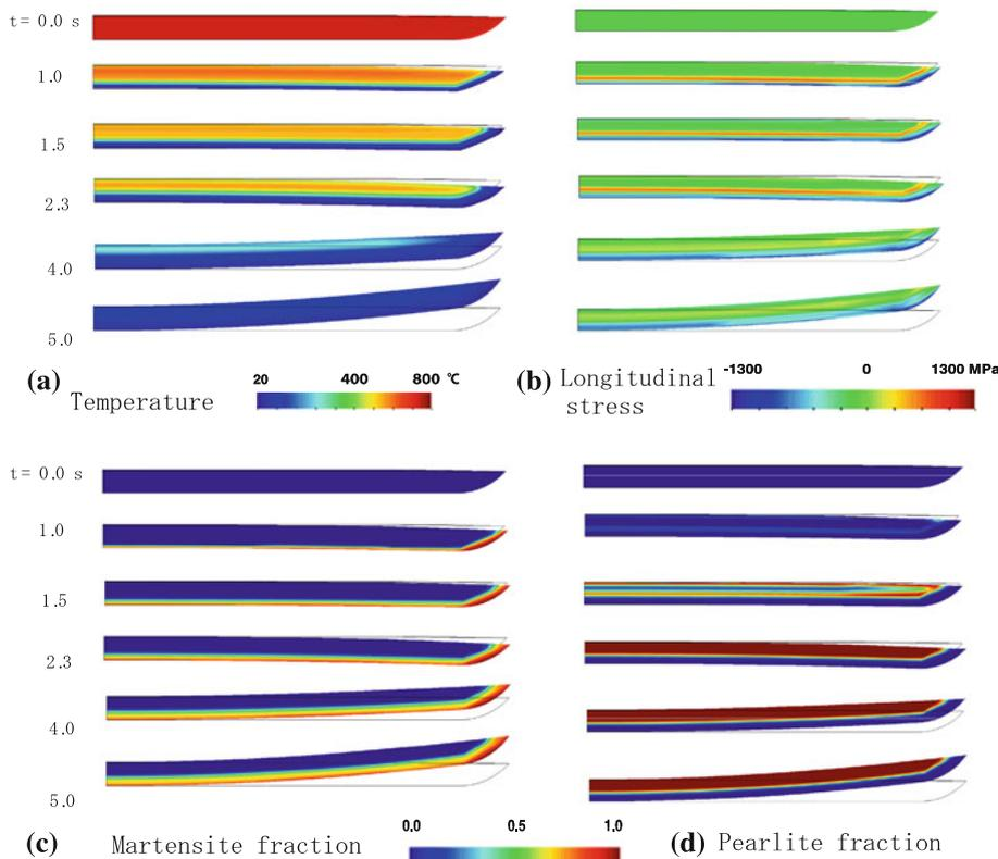
**Fig. 14** Simulated results of variation of temperature, stress and phase distribution with distortion
