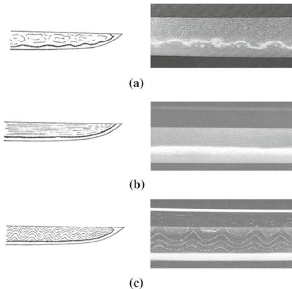
Fig. 5 *Hada*, weld patterns by forging with *hamon*, boundary of blade. **a** *Itame-hada*; **b** *Masame-hada*; **c** *Ayasugi-hada*
