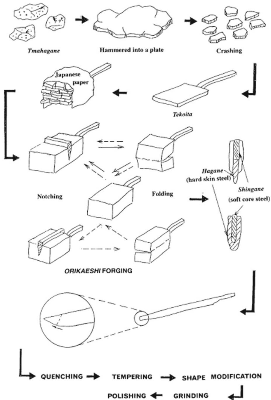
Fig. 3 Illustration of the manufacturing process of a Japanese sword
