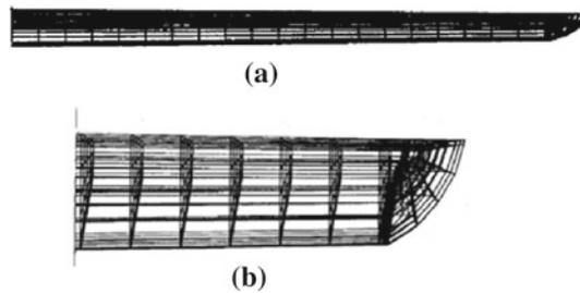
**Fig. 12** Finite element division of the sword. **a** Entire region; **b** Near the tip
