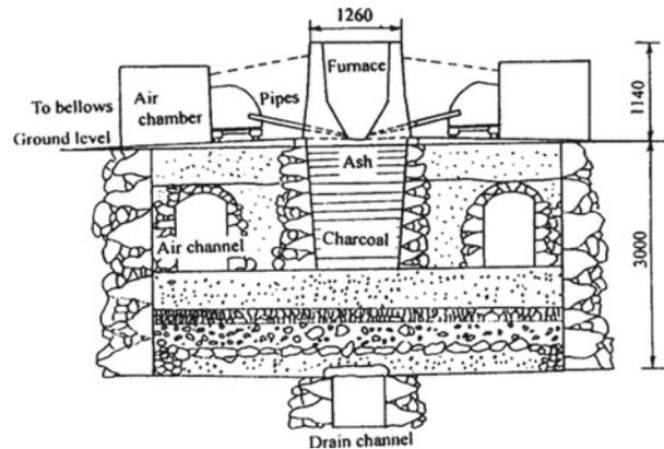
Fig. 2 Cross section of a *tatara* furnace
