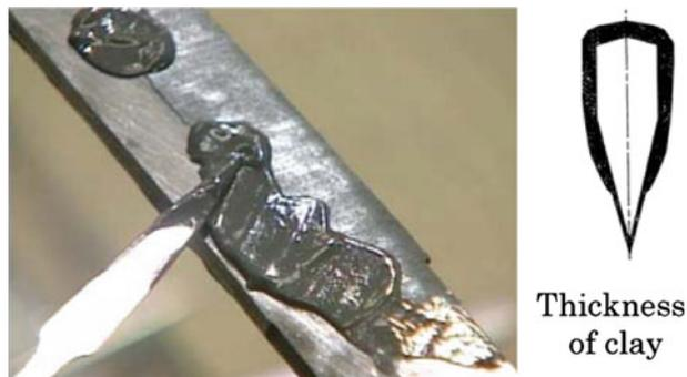
**Fig. 8** Clay coating technique
