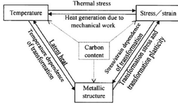
**Fig. 10** Coupling among metallic structures, temperature and mechanical fields in the course of the heat-treating process
