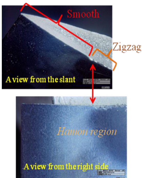
Fig. 9. Appearances of specimen after bending test and fracture surface (upper side: appearance from slant, lower side: one from side plane).
