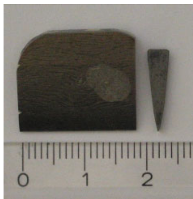
Fig. 1 Surface (left) prior to metallographic treatment and cross section (right) of the piece of the Damascus sabre investigated. The light spot on the surface is due to etching. Scale is in cm.
